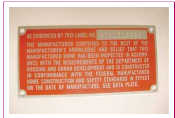
EXHIBIT 550.1 A HUD label required for mobile homes.
