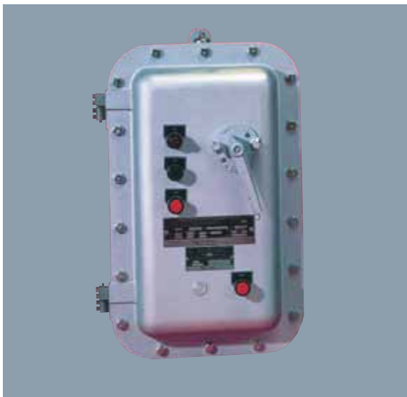
EXHIBIT 501.15 A magnetic motor starter for use in a Class I, Group D location. Note the number of securing bolts and the width of the flange. (Courtesy of O-Z/Gedney, Emerson Electric Co.)
