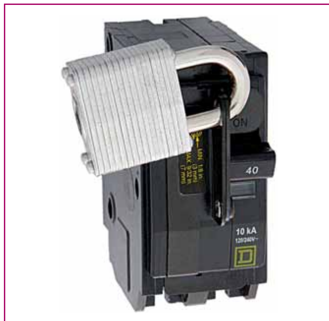
EXHIBIT 440.1 An example of locking hardware (with lock installed) that is not readily removable or transferable. (Courtesy of Schneider Electric)
