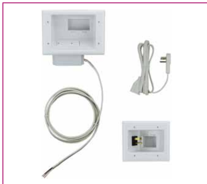
EXHIBIT 400.1 A listed assembly that includes an inlet, receptacle outlet, Chapter 3 wiring method, and a flexible cord. (Courtesy of DataComm Electronics, Inc.)
