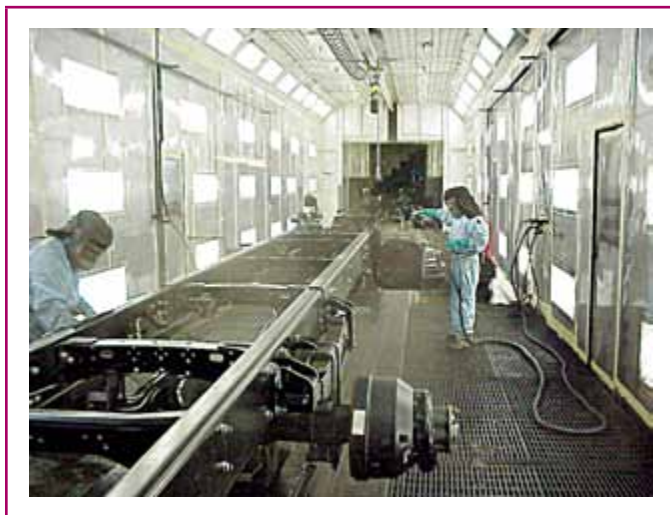
EXHIBIT 516.1 An enclosed paint spray room.
